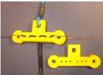
an ATU and my IC706. I made up a 3D printed central insulator for this antenna to test out the strength and UV stability of the plastics. It has been outside for six months and I have not seen any degradation so far. The antenna works well for the WADARC net and local as well as European contacts.
