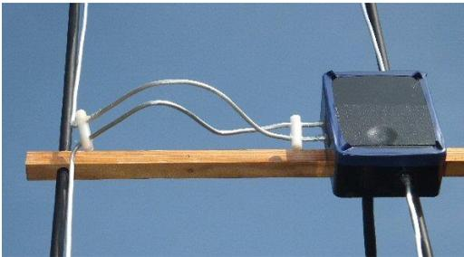
The three directors were made from aluminium rod (I used 3mm welding rod bought in a pack of 50 from EBay). I have a long length of 4mm diameter aluminium wire in my cupboard for years doing nothing so I used it to make the
