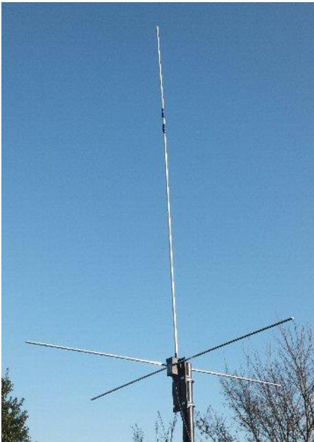
I made the 3D printed enclosure larger than the GP version so that it could take the matching coil. The coil can be adjusted for lowest SWR but in practice it is easier to adjust the length of the radiator. As with the GP antenna, once a good SWR has been achieved, the enclosure can be filled with sealant to weatherproof everything.
