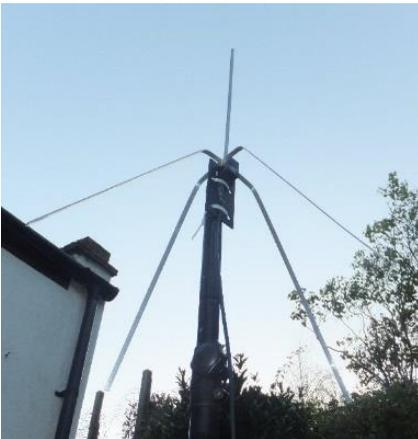
The four quarter wave ground planes are bent downward to produce a feed impedance of about  $50\Omega$  to match the coax.
